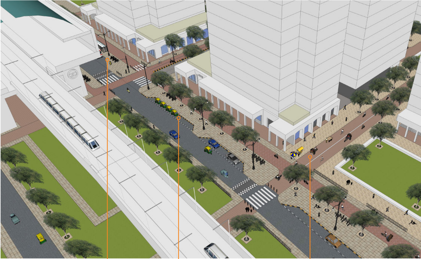
Grade-separated feeder service stop and access to station and connection to developments using non-motorized shared streets
