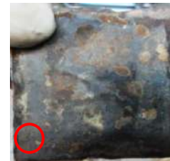
Anode with burn marks due to internal shorting
