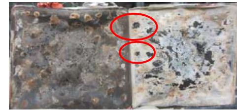
Circled areas show internal short circuit burns. In some cases, the short circuit burned completely through the separator
