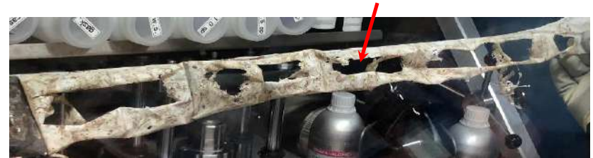
Separator burned through
