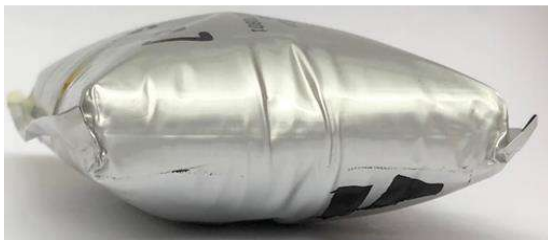
Swelling of damaged cell due to electrolyte decomposition due to overdischarge
