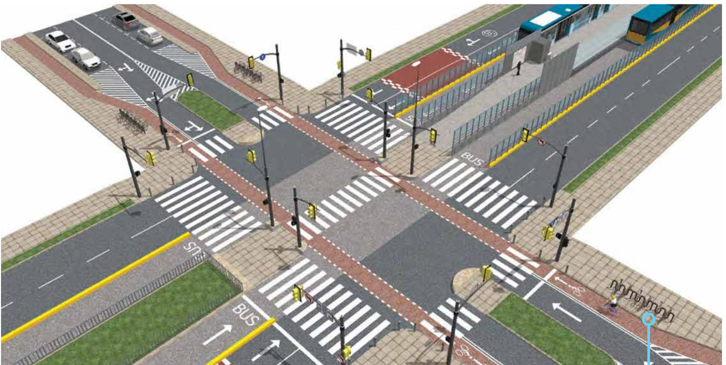
Cycle rack on sidewalk along the road perpendicular to the BRT lane, allowing riders to lock the cycles and transfer to BRT system.
