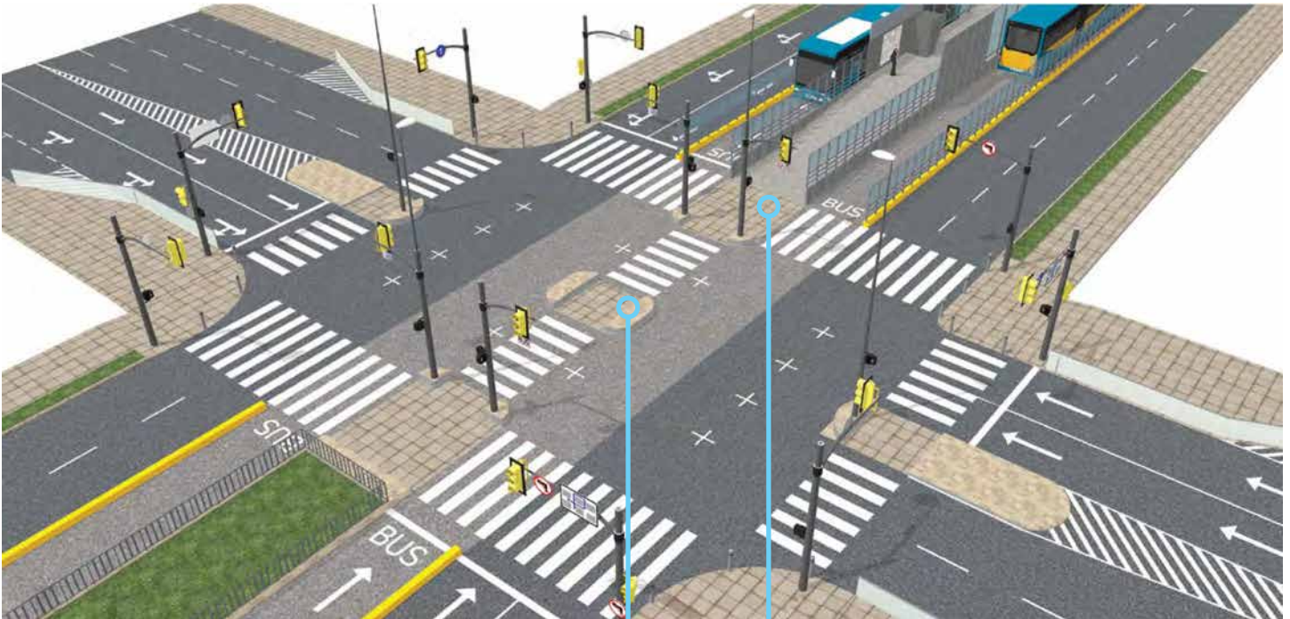
Pedestrians crossing along the median, especially with longer BRT Green phase.
