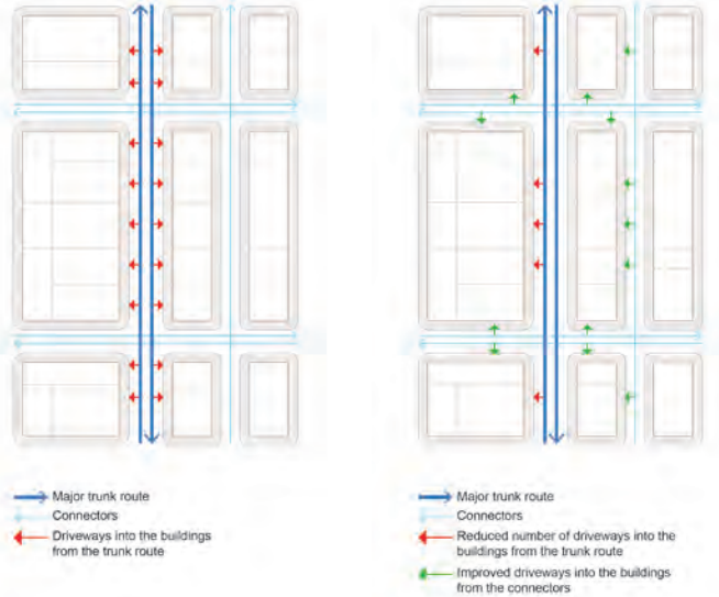
Existing conditions with driveways to buildings from trunk route. (Left), Reducing number of driveways into developments along the trunk route and providing entrances from connectors. (Right)
