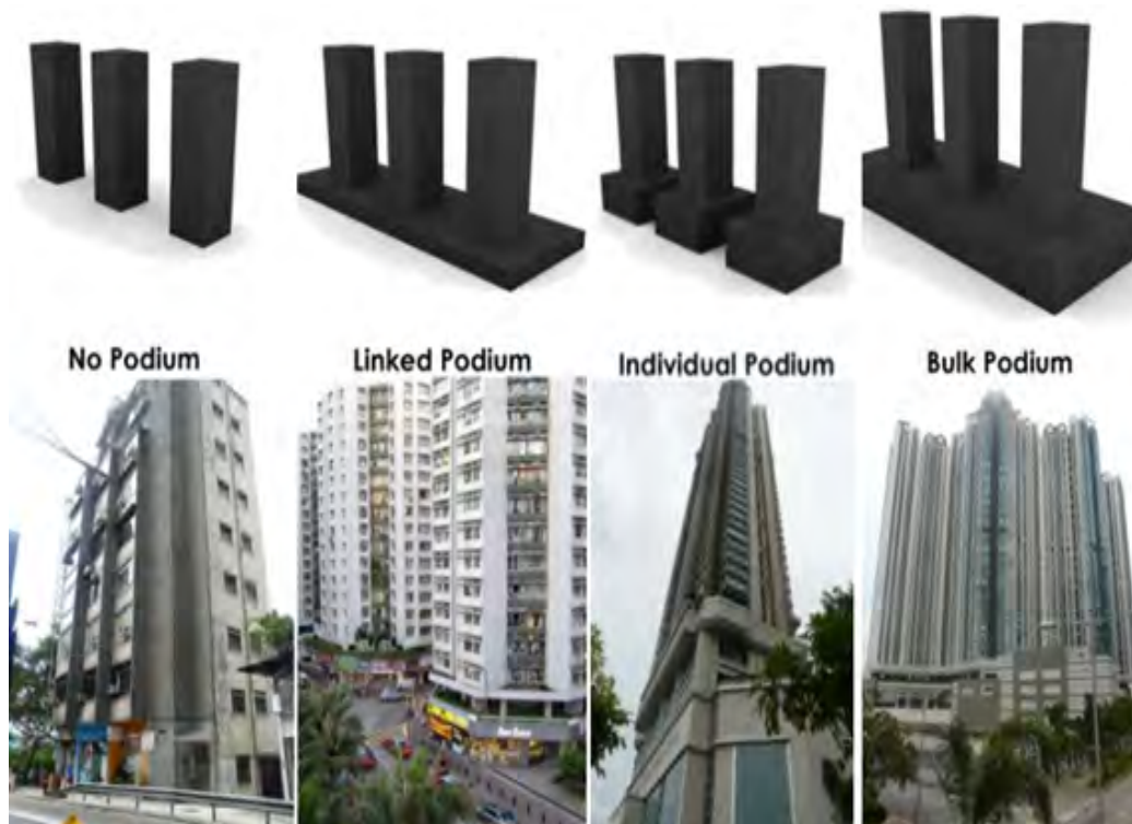
Figure 15: Podium Development Typologies in Hong Kong | Source: Dr. Sujata S. Govada ©UDP International. Reproduced with permission from Transport and Housing Bureau; further permission required for reuse.
