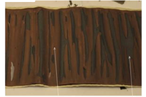
Cathode showed heavy copper plating Delaminated area, where active material was adhered to separator J. Nemanick et al., International Batt Seminar, March 2016
