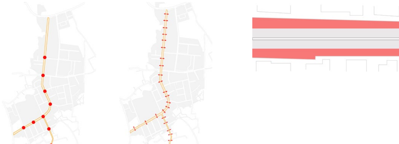
Figure 32 (left and middle) Raised intersections and pedestrian crossings; (right) consistent carriageway & reduced lane widths, Source: EMBARQ India
