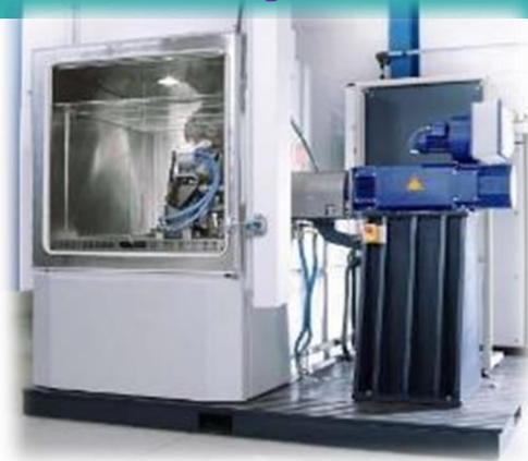
E-motor Test Bed 150kW and 250 kW
