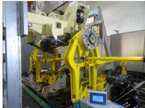
Evaluation of Battery Structure and supports using Multi-axis Shaker table "MAST".
