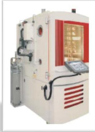
Environmental Chamber To Test Lithium-ion Cells Of Traction Battery
