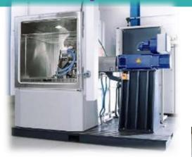
E-motor Test Bed 150kW and 250 kW
