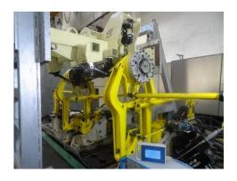
Evaluation of Battery Structure and supports using Multi-axis Shaker table "MAST".
