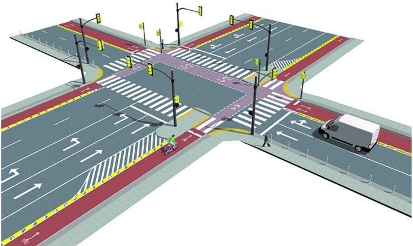
Concept drawing of an unprotected intersection.
