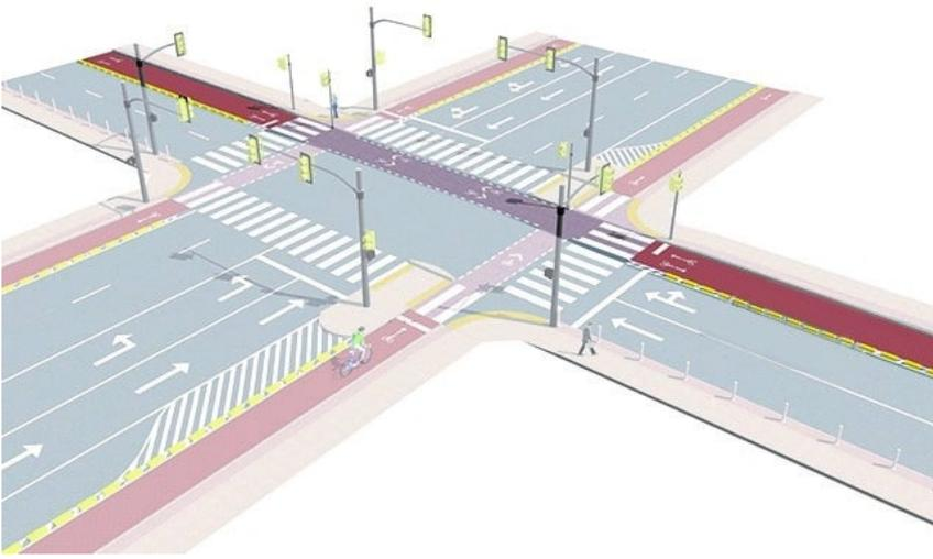
*Bi-directional protected lanes separated from car traffic through physical barrier.*
