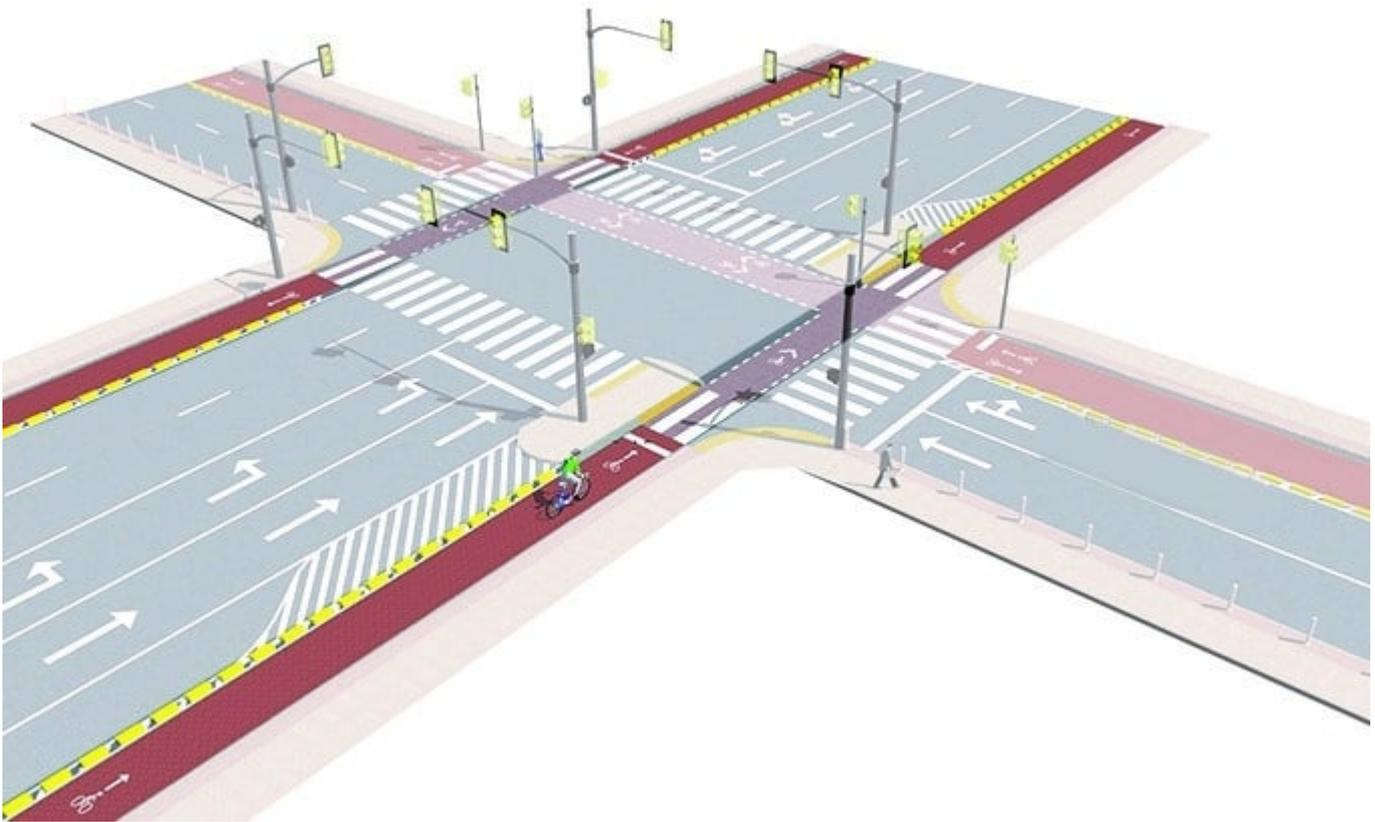
Uni-directional protected lanes separated from car traffic through physical barrier. Graphic by WRI.
