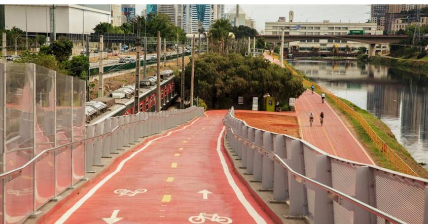
*Fig. 2: Example of lane markings that designate direction for*
