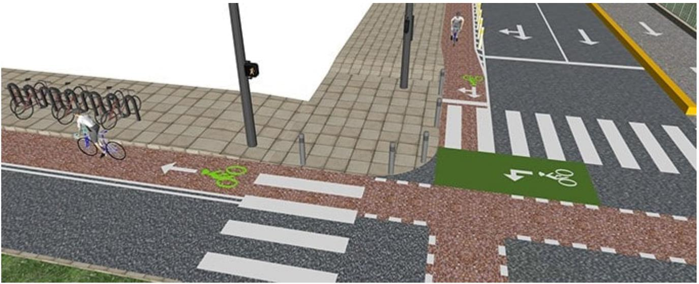
Concept drawing of an unprotected intersection.
